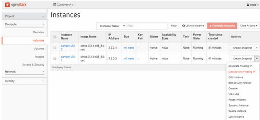
6. Select the + symbol to allocate a floating IP from an existing external network, then click **Associate**.
