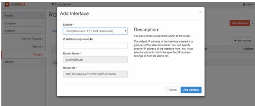
The interface is now attached to the router, as shown in the following example.
