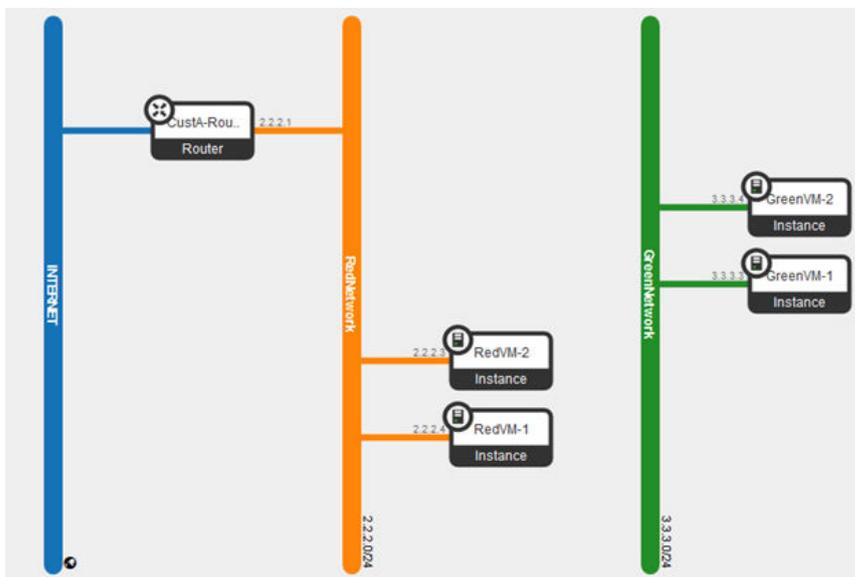
The following example shows VM and floating IP details for Customer A.
